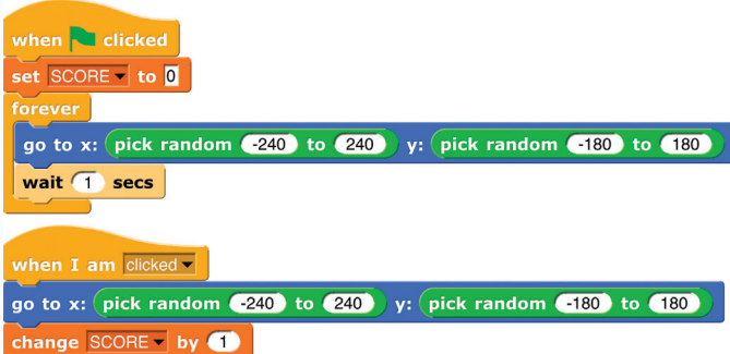
Figure 3: The Snap! code for the “Whack Alonzo” mobile app, which can be written in 60 seconds, and loaded on a mobile device in only 30 more seconds.
